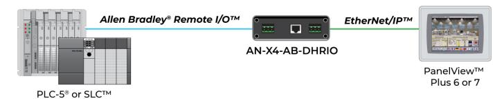
This operating mode allows legacy PanelViews to be upgraded to a PanelView Plus 6 or PanelView Plus 7 via EtherNet/IP.
