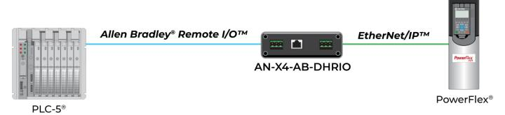
This operating mode supports upgrading legacy Allen Bradley drives on Remote I/O to new EtherNet/IP-enabled drives.
